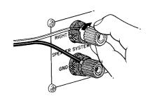
**CAUTION**: Two speaker systems can be connected to this unit. The minimum speaker impedance should be 4 Ohm when only one speaker system is connected. When two speaker systems are connected, care should be taken that net impedance does not become less than 4 Ohm.
